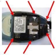
Screw 6 self taping screws torx 6 with a manual screwdriver
