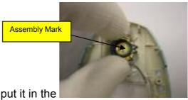
Take an earpiece. Remove the protection foil and put it in the front. ( Take care to the earpiece orientation )
