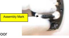
Take a gasket ,insert the gasket on the Lumberg door (Take care to the gasket orientation )
