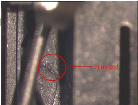
Lock mechanism damaged
