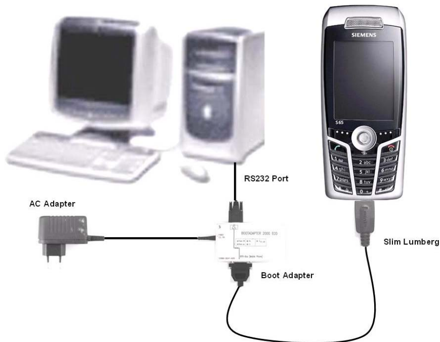
Figure 1. S65 / SP65 Software Programming Setup
