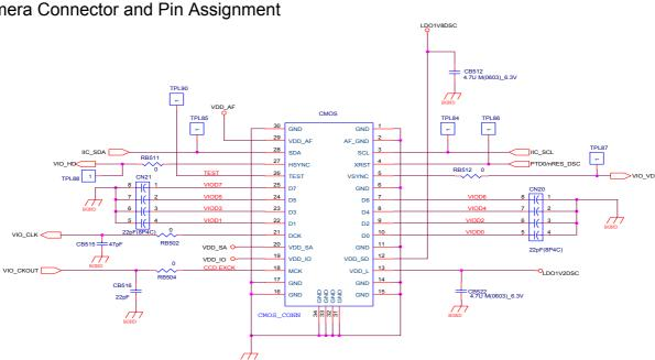
Camera Connector and Pin Assignment
