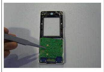
Remove Keypad MMI by using Tweezers carefully.
