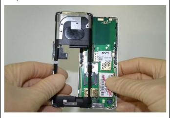
Assemble Lower Case onto the Upper Case.
