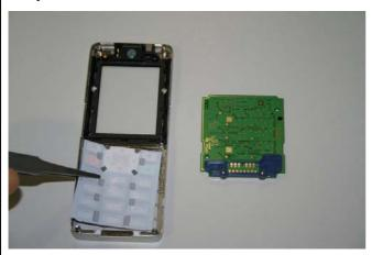
Remove Keypad by using Tweezers carefully.
