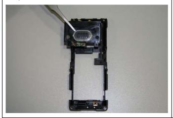
Assemble Ringer by using Tweezers.
