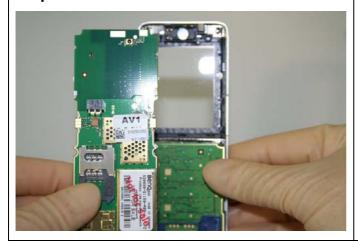
Place PCB with assembled Display in the Upper Case.
