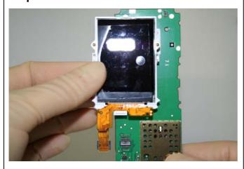
Assemble Display Module on PCB.
