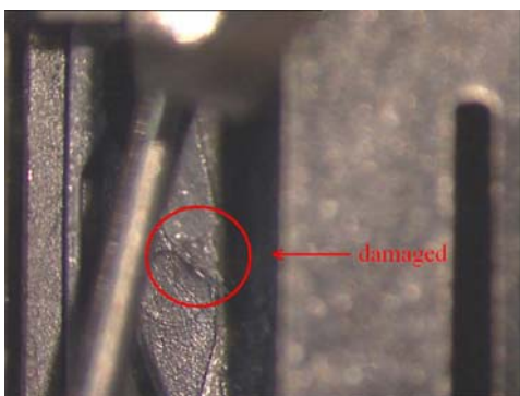
Lock mechanism damaged
