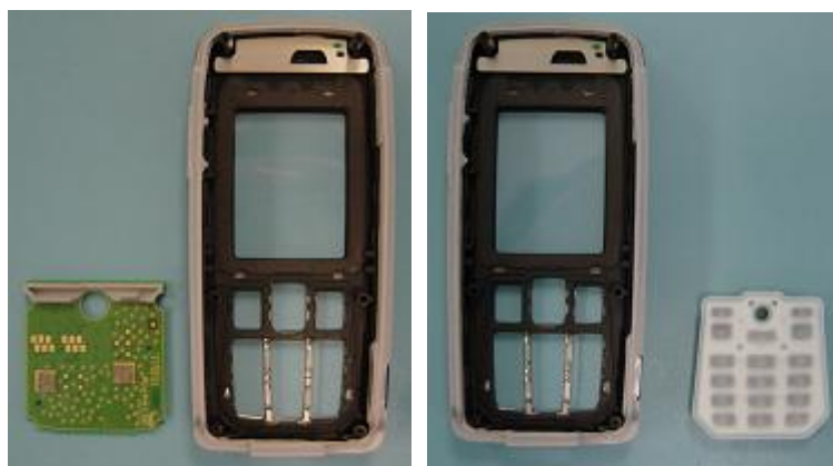
Remove MMI and Keypad
