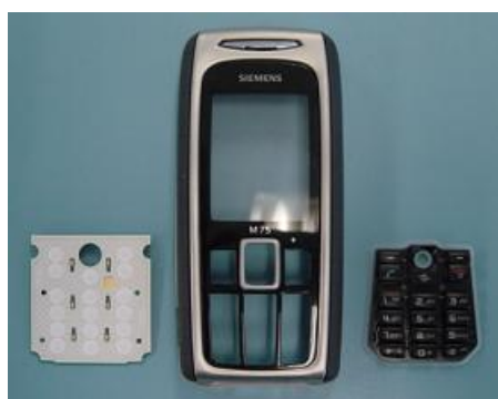
Remove MMI and Keypad
