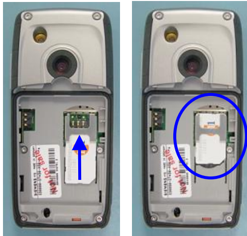
Installation of the SIM card
