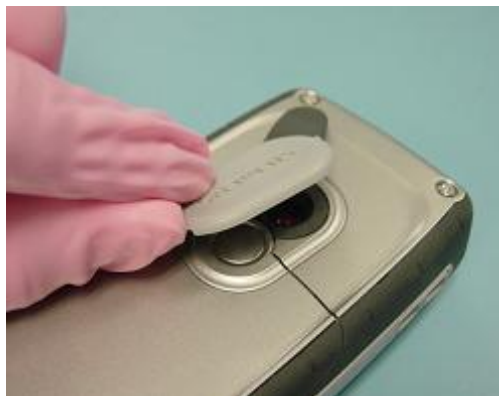
Remove Camera lens cover
