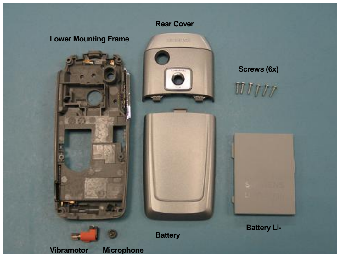
Fully disassembled CX75 - upper parts (top) and lower parts (bottom).
