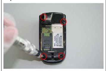
Remove screws by using the Torque
