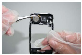
Remove the Ringer by using Tweezers carefully.
