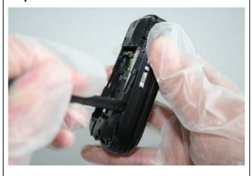
Remove Lower Base Case Shell by using the Alternative Opening Tool.
