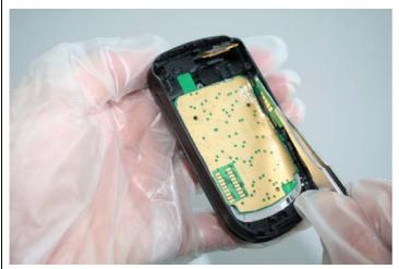
Assemble the Side Key PCB by using Tweezers.
