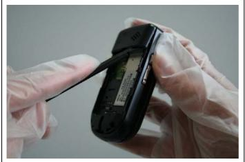
Remove Rear Cover by using the Alternative Opening Tool carefully.
