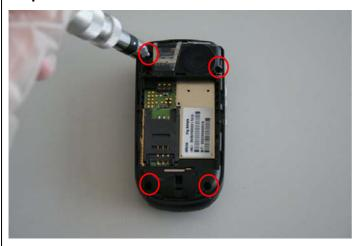
Place screws by using the Torque – Screwdriver T5+.
