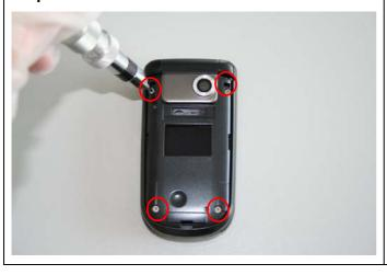
Remove Screws by using the Torque
