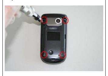
Place screws by using the Torque – Screwdriver T5+.
