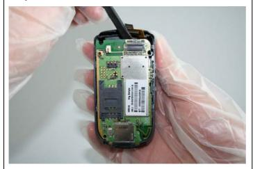
Remove the RF Control Board by using the Alternative Opening Tool carefully.
