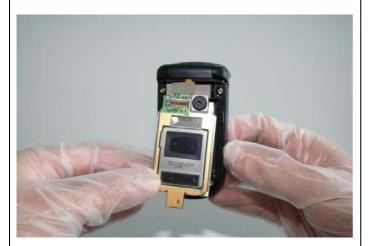
Assemble the Display Module.
