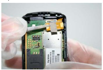
Connect the Flex Cable with the socket.
