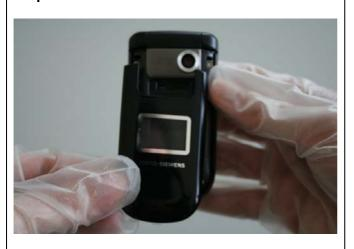
Assemble the Lower Lift Case Cap.
