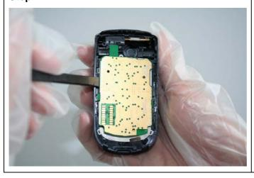
Remove the Keypad PCB.
