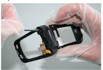
Use the Hinge Tool very carefully to remove the Upper Base Case Shell from the Lower Lift Case Shell.
