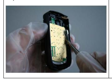
Assemble the Side Key Left by using Tweezers.
