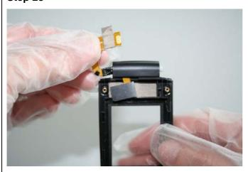
Remove the Flex Cable carefully.
