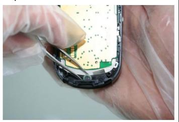
Remove the Microphone by using Tweezers. Take care of the spring contact.
