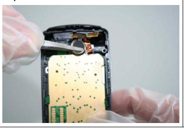
Assemble the Vibra-Alert by using Tweezers.
