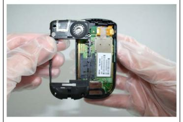
Assemble the Lower Base Case Shell.
