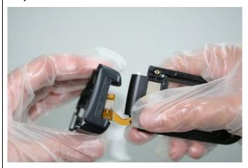
Insert the Flex Cable into the Lower Lift Case Shell.
