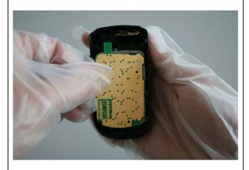
Assemble Keypad PCB.
