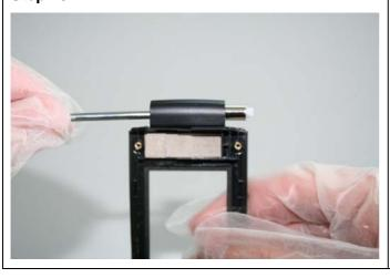
Remove the Hinge by using the Hinge Tool.
