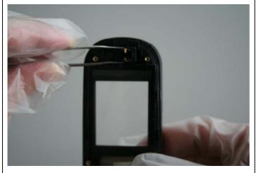
Assemble the Earpiece by using the Tweezers.
