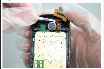
Remove the Vibra-Alert by using Tweezers.
