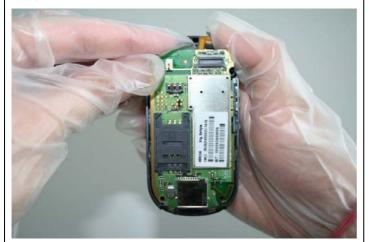
Assemble the RF Control Board.
