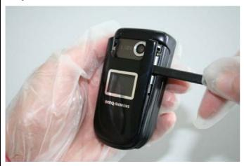
Remove Lower Lift Case Cap by using the Alternative Opening Tool carefully.
