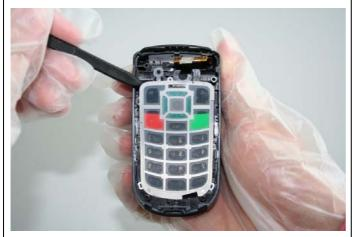
Remove the Keypad by using the Alternative Opening Tool.
