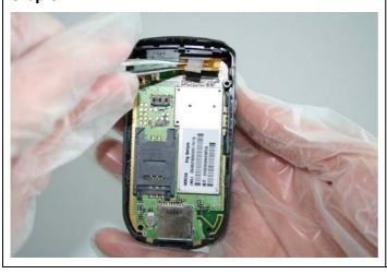
Disconnect the Flex Cable by using Tweezers.
