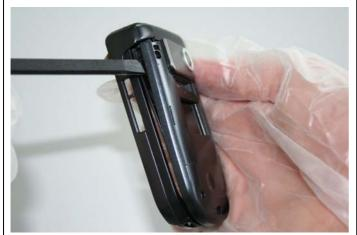
Remove Upper Lift Case Shell by using the Alternative Opening Tool carefully.
