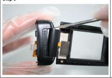
Assemble the Lower Lift Case Shell and the Upper Base Case Shell by using the Hinge Tool.
