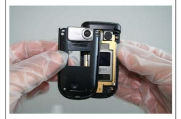
Assemble Upper Lift Case and Lower Lift Case.
