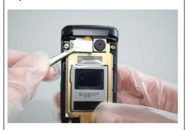
Connect the Flex Cable with the socket.
