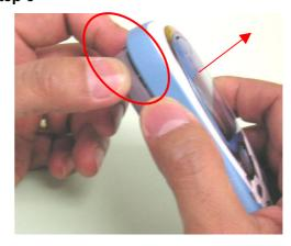
To remove the CLIPit cover, gently pull the cover upwards from the side of the phone while holding firmly the lower mounting frame as shown.
