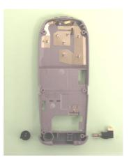
Remove the Vibrator motor and MIC from the Lower Mounting Frame.
