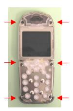
To remove the SAR frame and Light Guide assembly from the lower mounting frame, unscrew the 6 screws (as indicated) with a T5 Plus screw driver (set Torque = 16 cNm).
