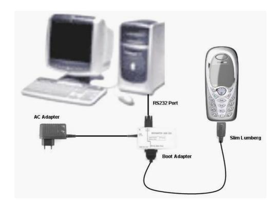
Figure 1. C60 Software Programming Setup
