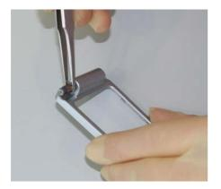
Push the Hinge inside the Frame.
