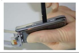
Remove Front Cover with the Alternative Opening Tool.
