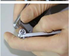
Remove Upper Case from Lower Case by pushing the Hinge-spring, now you can separate the Upper Base Frame from the Lift Frame.
