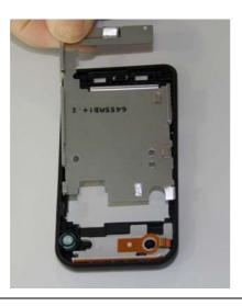
Assemble PCB cover plate.
