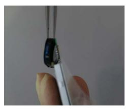
Disconnect the loudspeaker from PCB with Tweezers.
