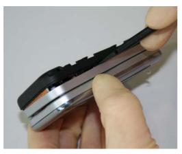
Remove rear cover with the Alternative Opening Tool carefully.
