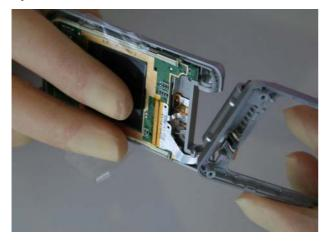
To assemble the Display, you have to push the Flex Cable through the slot of the Lift Cover.
