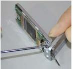
Use the Hinge – Tool to push the Hinge spring inside to assemble the Upper Case with Upper Base Case.
