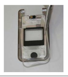
Assemble Display Spacer.
