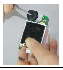
Assemble mircrophone by using tweezers.
