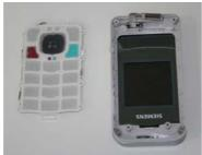
Remove Keypad by using Tweezers.
