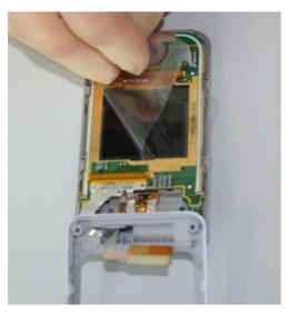
Attention! Before assembling the Display Module it is mandatory to remove the Display Foil!
