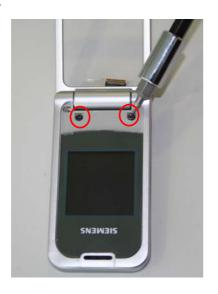
Remove screws with the Torque – Screwdriver T5+
