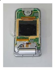
To avoid scratches it is mandatory to place a protection foil onto the Display!!!
