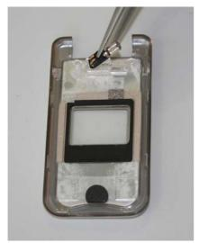
Remove Vibramotor by using tweezers.
