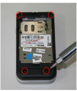
Remove screws with the Torque – Screwdriver T5+
