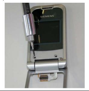
Fix screws with the Torque – Screwdriver T5+
