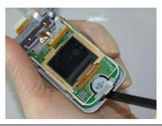
Remove PCB by using the alternative opening tool. Separate Earphone from front cover carefully.
