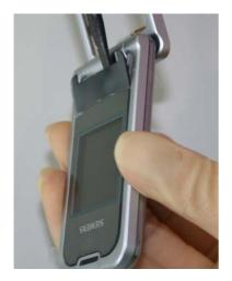
Remove screw cover by using the alternative opening tool carefully.
