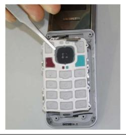
Assemble the Keypad by using Tweezers.
