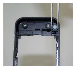
Remove microphone by using tweezers carefully.
