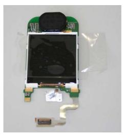
To avoid scratches it is mandatory to place a protection foil onto the Display!!!
