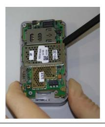
Assemble PCB by using the tweezers carefully.
