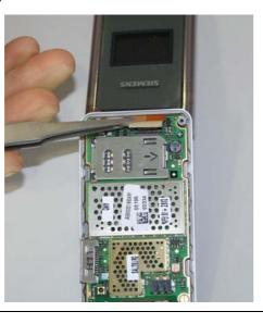
Connect the Flex Cable with the assembled PCB.
