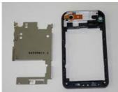
Remove PCB cover plate by using the alternative opening tool.
