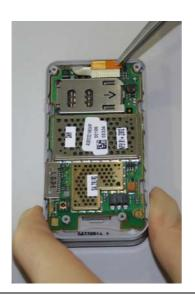
Disconnect the Flex Cable from PCB by using Tweezers.
