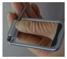
Remove Hinge - Spring by pushing it through the Hinge.
