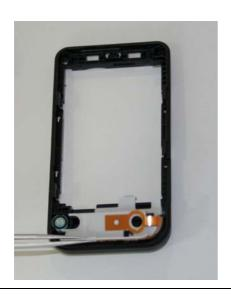
Assemble antenna module by using tweezers.
