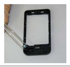
Assemble microphone by using tweezers.
