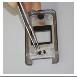
Assemble Vibramotor by using tweezers.
