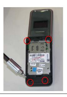
Place screws with the Torque – Screwdriver.
