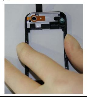
Remove antenna by using the alternative opening tool.
