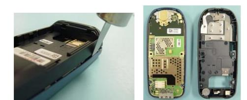
Remove Lower mounting frame with Vibra and Micro.
