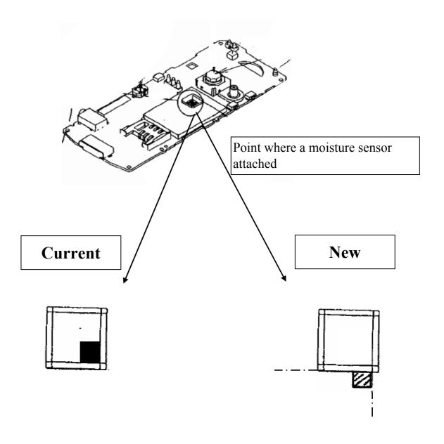
Notice) Board units include keyboards and it is compatible with one another on a unit basis, so you are not allowed to exchange only boards or keyboards between old and new board units.
