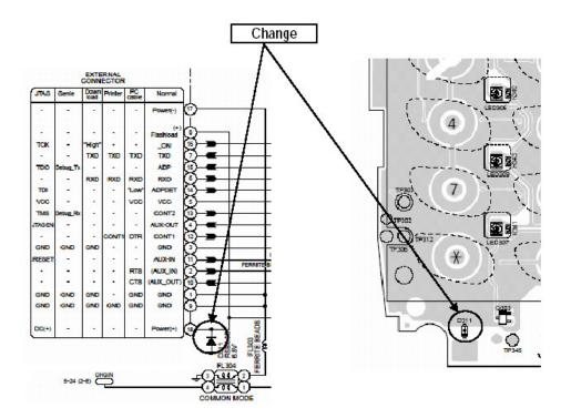
It is not necessary to replace the diode unless it is found to be faulty.
