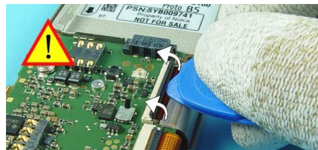
38.) Unlock the flex connector with SRT-6 carefully.
