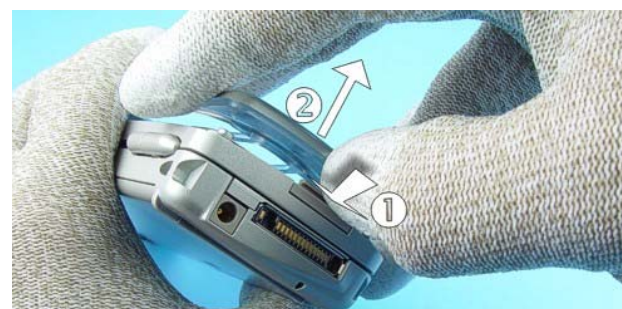
5.) Push the Latch and open the A-Cover Assy .
