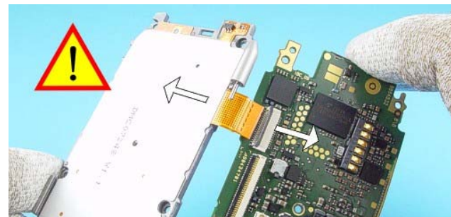
Remove the flex from the connector carefully.
