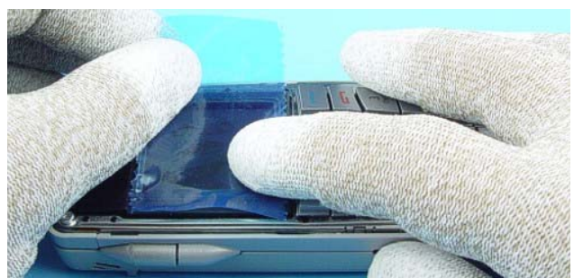
6.) Protect the LCD Module with a film.
