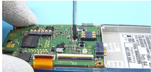
Unscrew the Torx Plus® size 6 screw.
