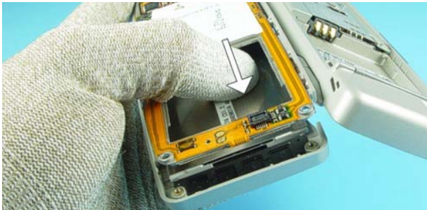
21.) Press out the C-Cover Assy carefully.
