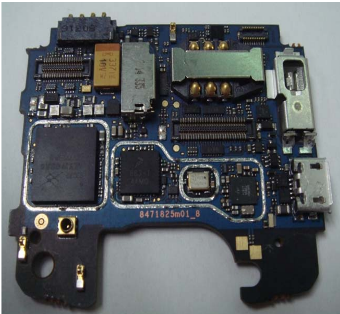
Photograph 9-1: Front side view of radio PC Board, without shields.
