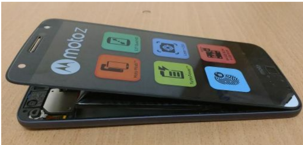
Figure 1.0 - Swollen Battery Condition
