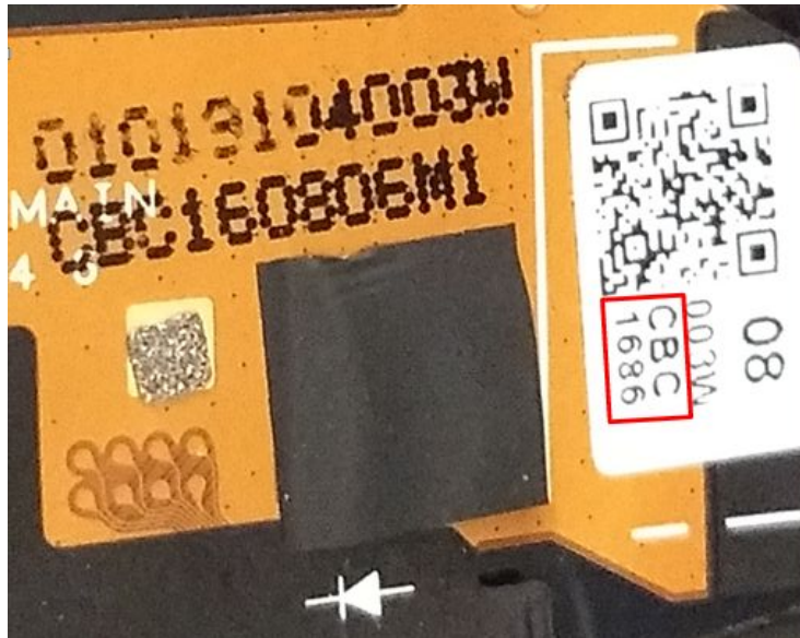
Figure 2.0 - Display Flex 8S Label Revision Marking: First character F or later = (CBC to FBC) Date Code Marking: YYMMDD = (16125 = 12/5/2016)
