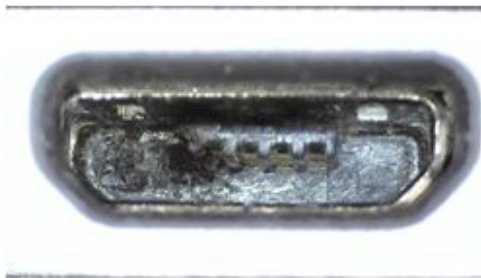
Fig. 2a - External Contact Damage
