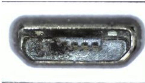
Fig. 2a - External Contact Damage
