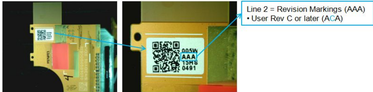
Figure 2 - Revision Part Marking Location (Rev A Shown)
