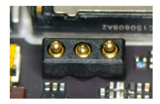
Cross-Section of the affected pin of the Pogo-Pin Connector M5760 (p/n: 39014039007) determined that the diameter of the barrel was slightly undersized, due to a supplier process issue.
