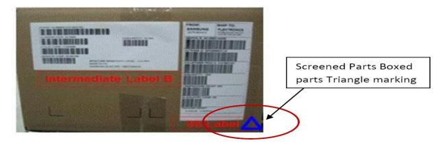
**Note:** Screened part boxes are marked with triangle as shown in photo above.
