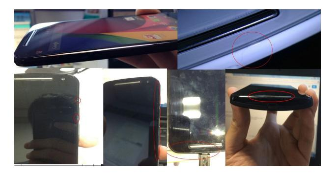
Engineering analysis root caused this issue to a manufacturing process issue when assembled the touch panel.
