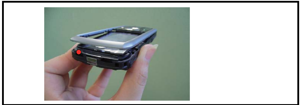
Figure 8. Removing the Front Housing
