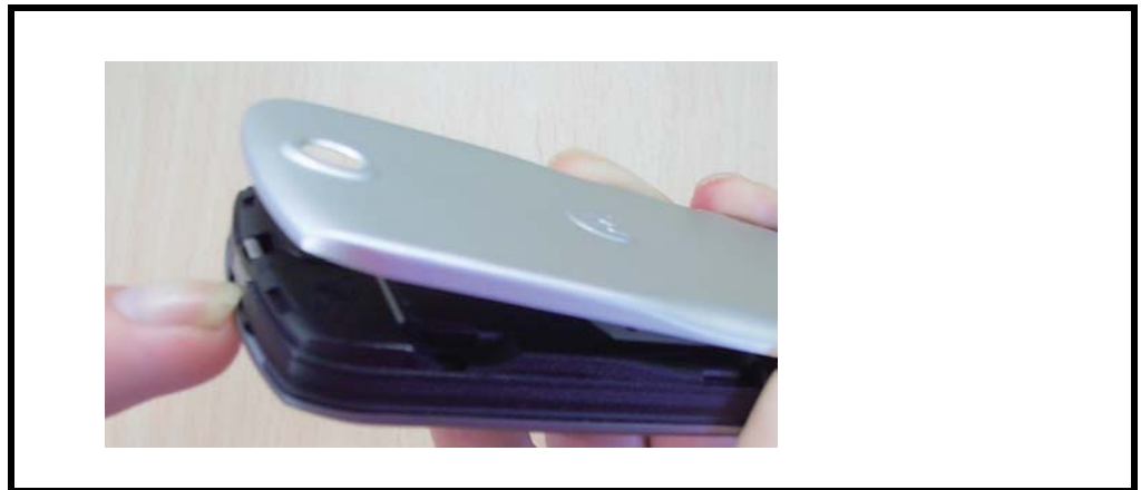
Figure 4. Removing the Battery Cover
