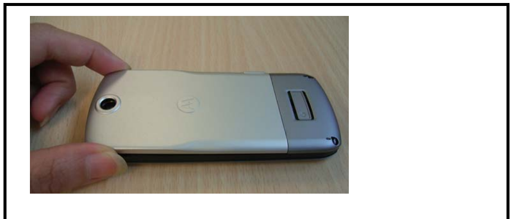
Figure 5. Replacing the Battery Door
