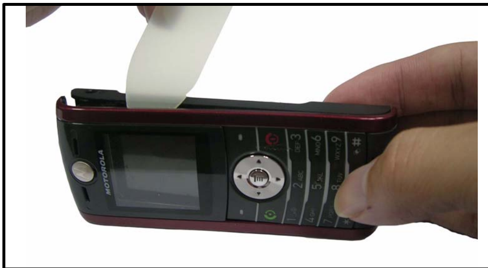
Figure 10. Prying the case apart along the seam
