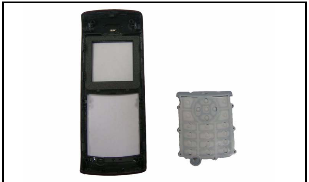
Figure 12. Removing the rubber keypad
