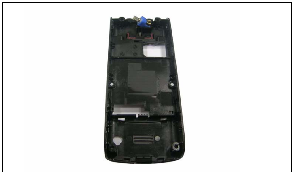
Figure 14. Removing the vibrator module
