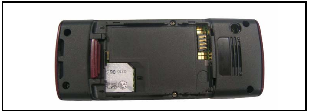
Figure 7. Removing the SIM card
