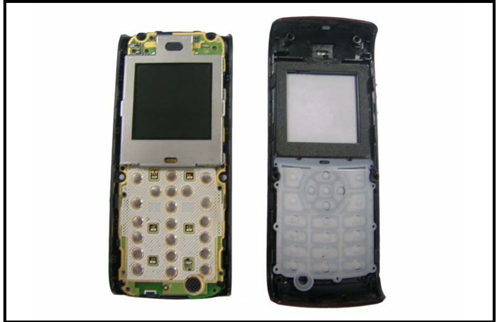
Figure 11. Removing the front housing
