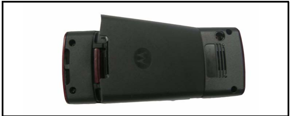
Figure 5. Removing the battery cover
