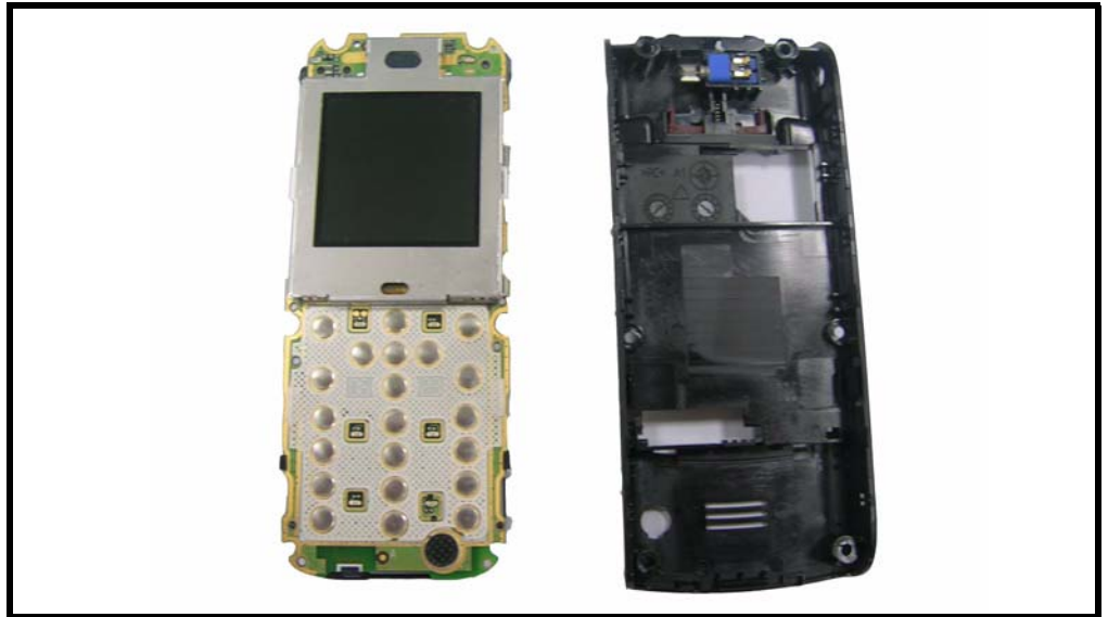
Figure 13. Disengaging the side hooks
