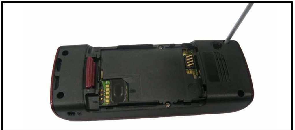
Figure 8. Removing the six T5 screws
