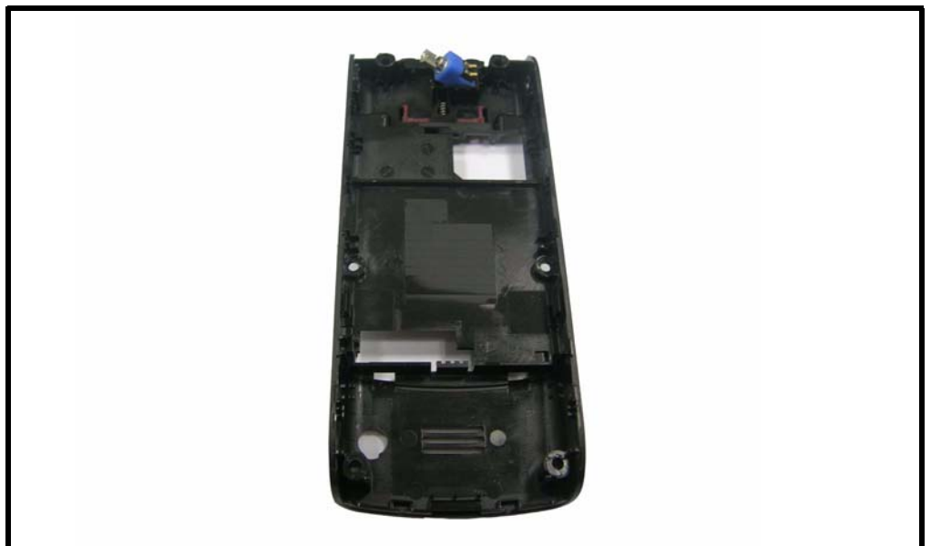
Figure 14. Removing the vibrator module
