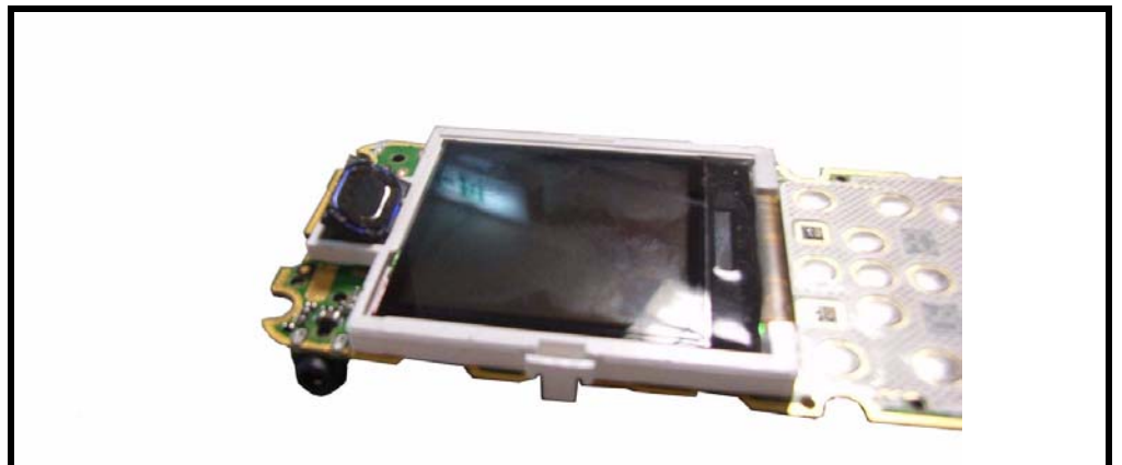
Figure 20. Pop out the receiver
