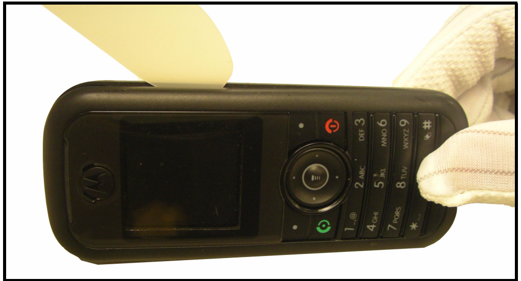
Figure 9. Prying the case apart along the seam
