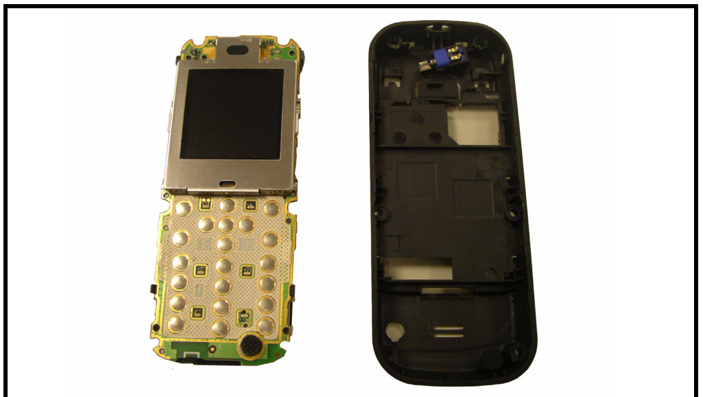
Figure 12. Disengaging the side hooks
