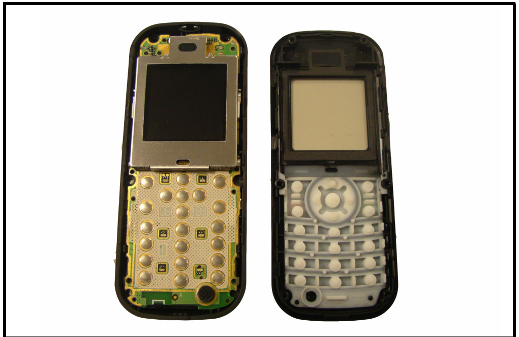
Figure 10. Removing the front housing
