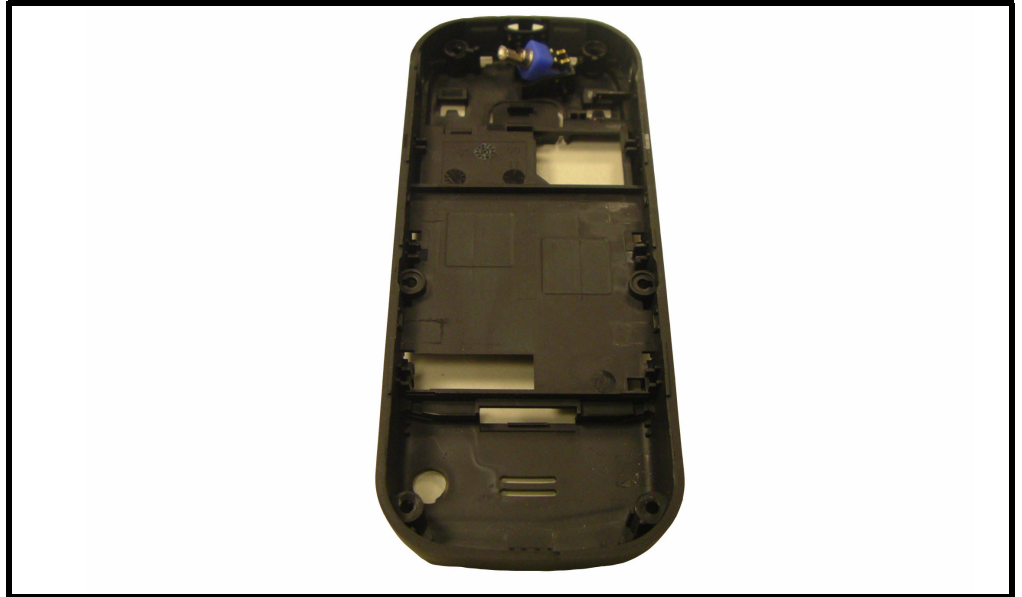
Figure 13. Removing the vibrator module
