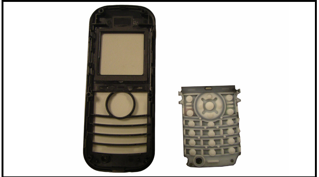
Figure 11. Removing the rubber keypad
