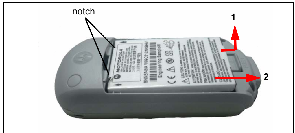
Figure 7. Removing the Battery
