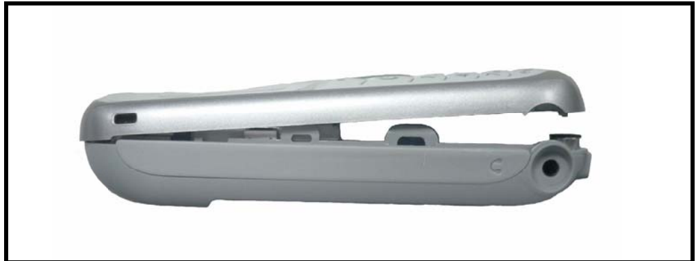
Figure 11. Remove the front housing
