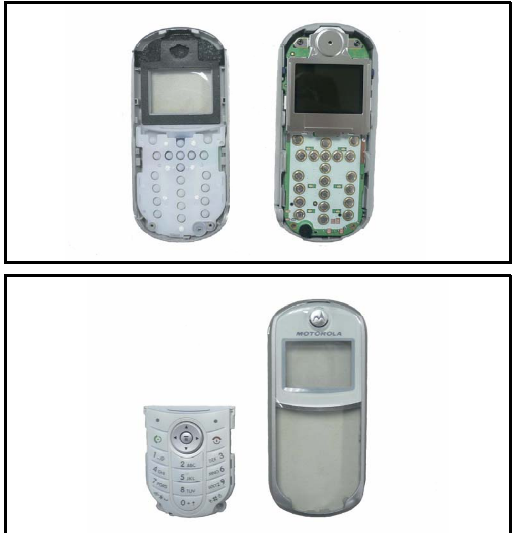
Figure 12. Remove and replace the rubber keypad
