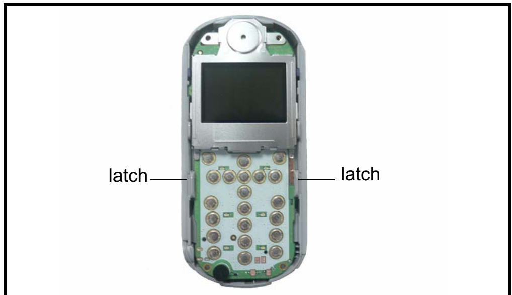
Figure 14. Pry open the side latches securing the Transceiver board to the back housing
