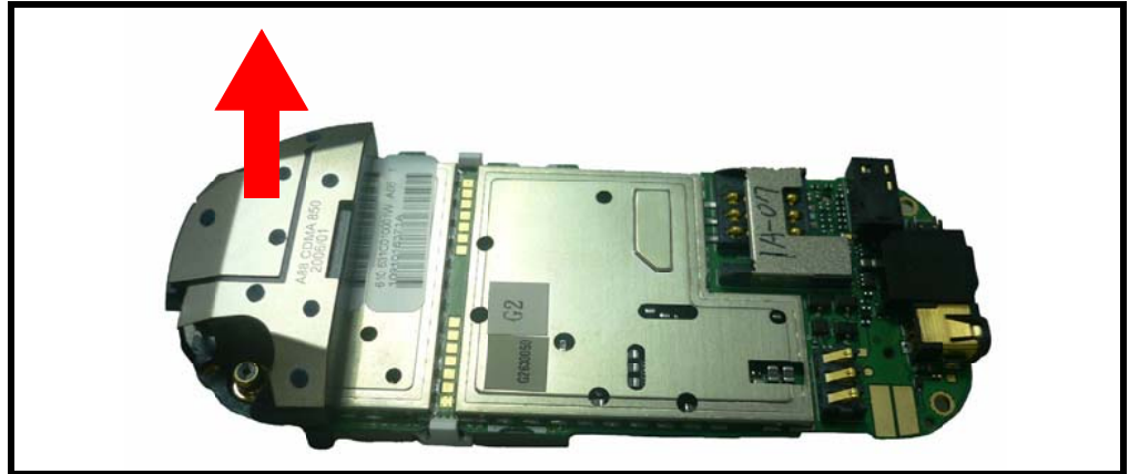
Figure 16. Gently off the antenna module from the Transceiver board
