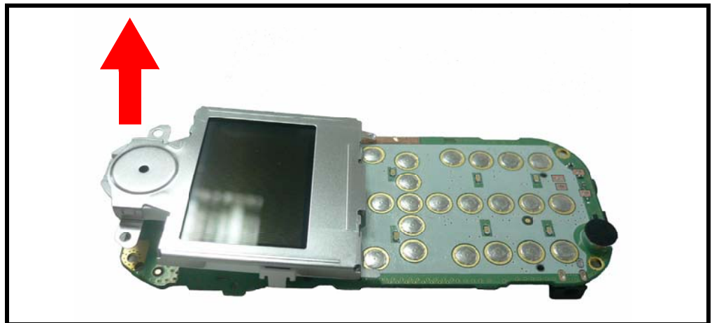
Figure 17. Pry the LCD screen away from the Transceiver board
