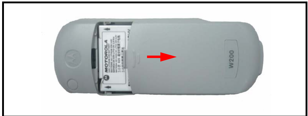
Figure 6. Removing the Battery cover
