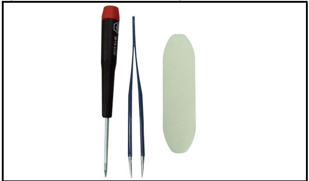
Figure 5. A screwdriver (T5), a pair of tweezers, and a wedge tool
