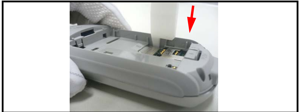
Figure 10. Use a flat wedge tool to pry the case
