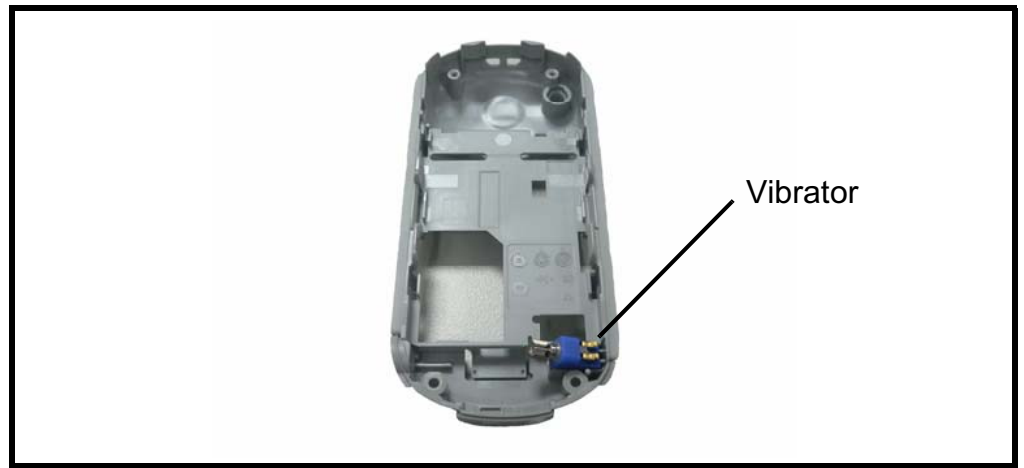
Figure 15. Gently pry up the vibrator motor on the inside of the back housing
