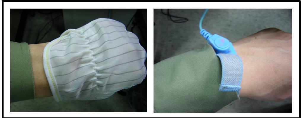
Figure 4. Antistatic wrist band and Antistatic glove
