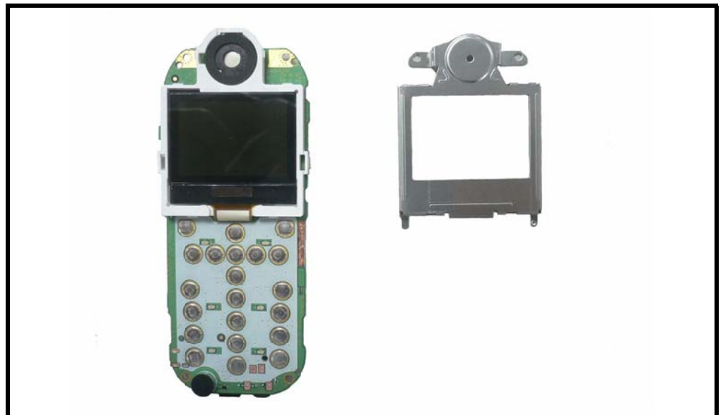
Figure 19. Removing LCD shielding case
