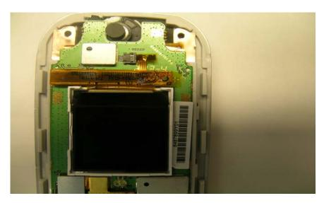
During Reassembly of flip, Flip screws should have  $1.5 \pm .01$  in-lbs of torque applied.
