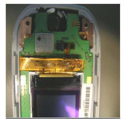
Step 2: Fold CLI flex assembly carefully as shown
