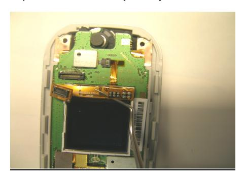
Step 3: Disassemble CIF flex from CIF connector
