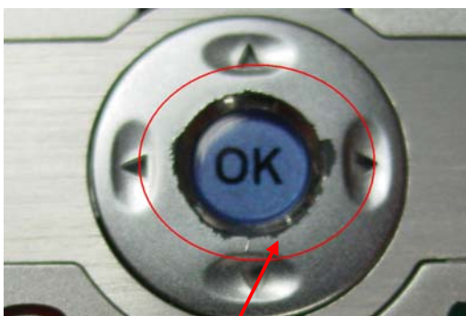
Paint Peel Off
