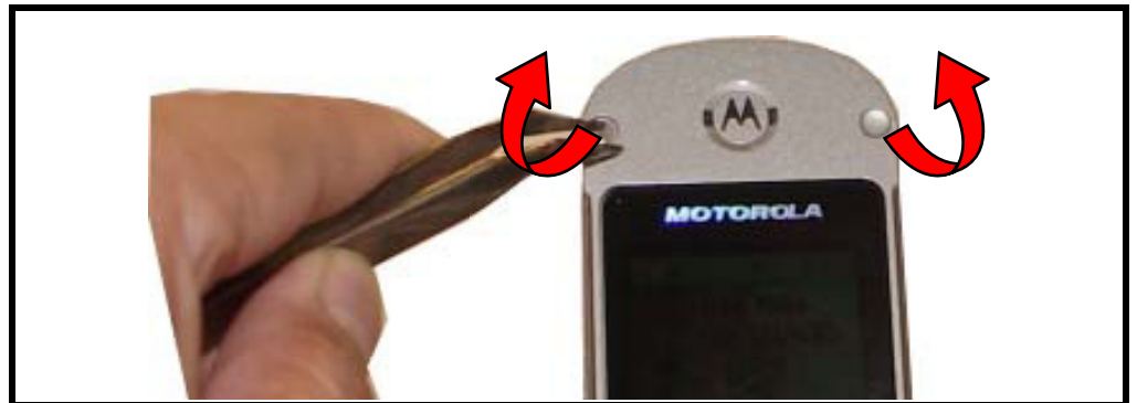
Figure 14. Removing the Flip Assembly Screw Caps
