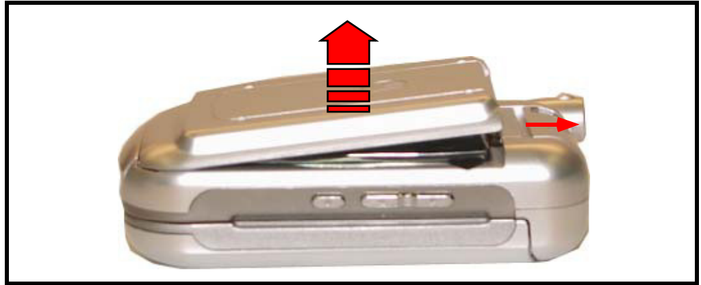
Figure 4. Removing the Battery Cover
