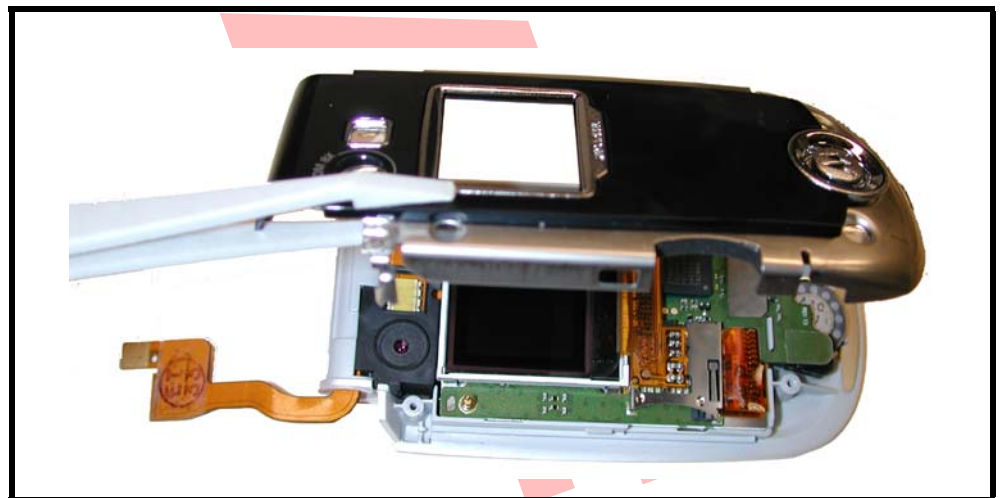
Figure 18. Removing the CLI Lens Assembly
