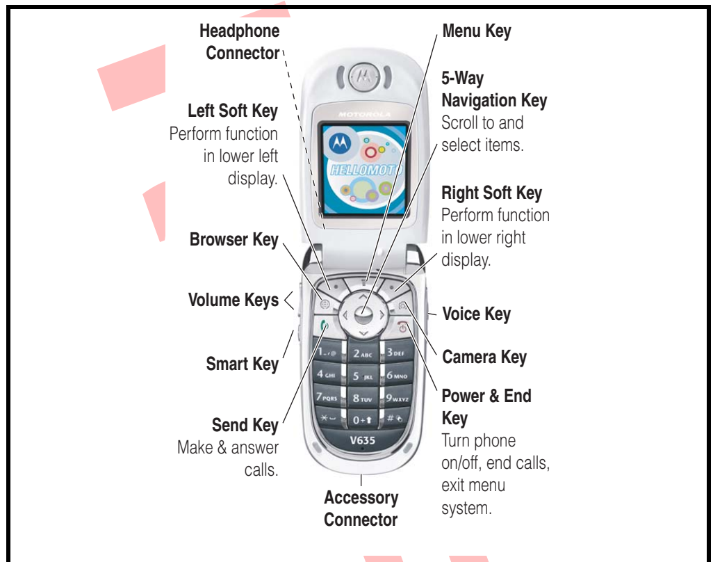
Figure 1. Telephone Controls, indicators, and I/O
