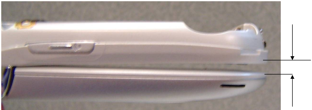
Fig. 1.0 - Flip falls away from base, creating a gap between the flip and base bumpers
