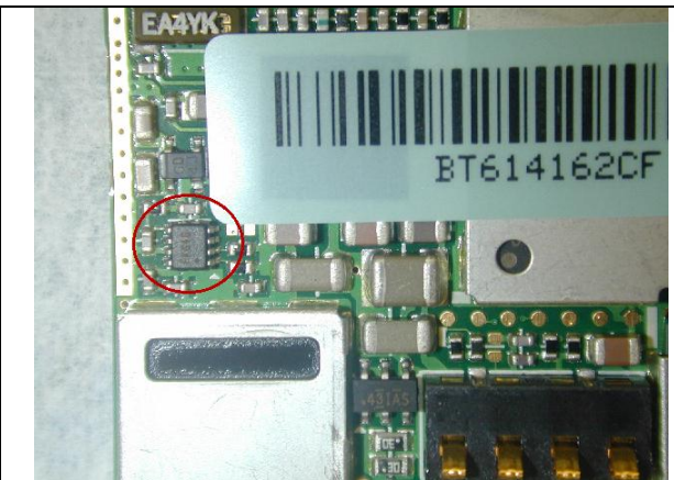
Figure 2. V510 and V810. IC303 is highlighted.
