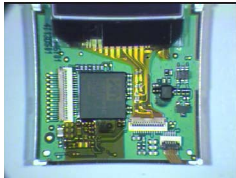
Fig. 2.0 - Kapton Tape (1190142N01) Dimensions: 13.0mm x 8.5mm, 0.08mm thick
