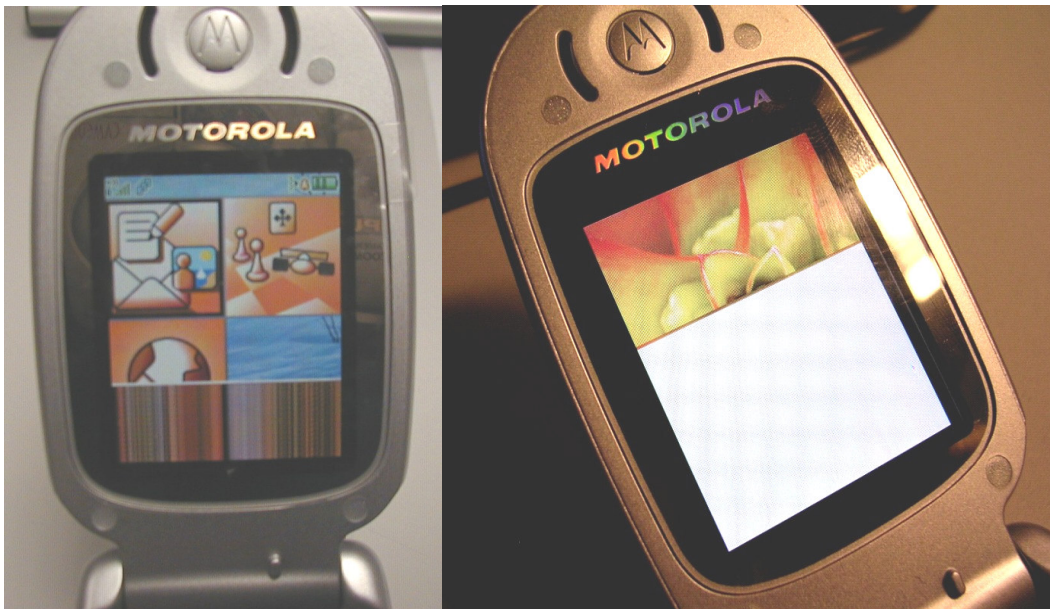
Figure 1.0 – SEC TMR Display with Gate-Block Failure
