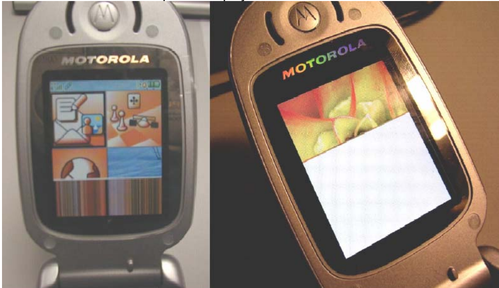
Figure 1.0 – SEC TMR Display with Gate-Block Failure
