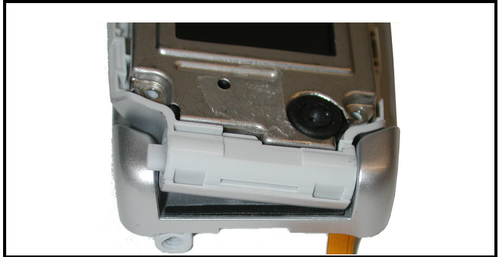
Figure 16. Reinserting the Flip Assembly
