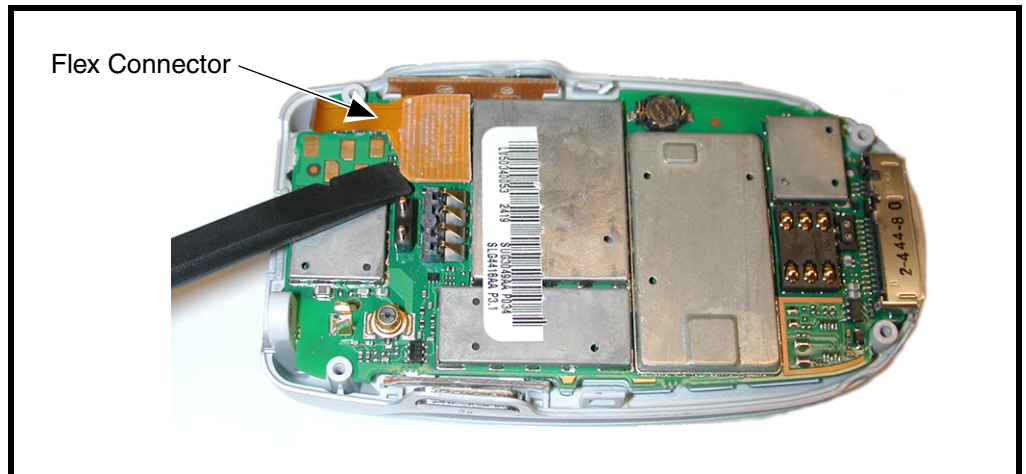
Figure 8. Disconnecting the flex from the transceiver board
