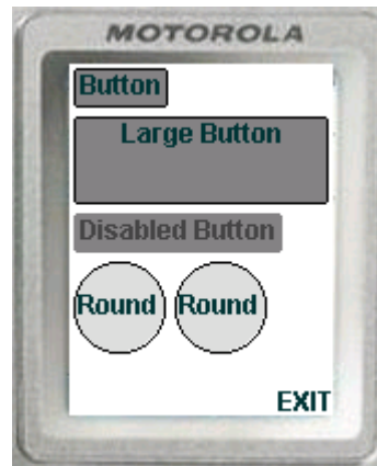
Figure 23. The second round button, positioned relative to the top and right edge of the first round button.
