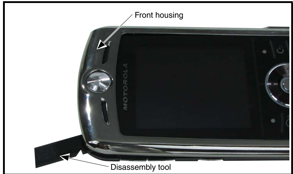
Figure 14. Releasing the Front Housing Catches
