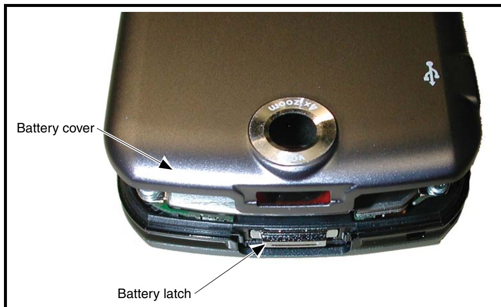
Figure 3. Removing the Battery Cover
