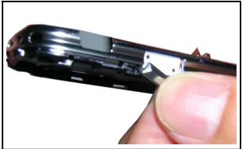
Figure 15. Removing the Side Key
