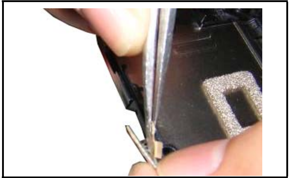
Figure 20. Removing the Adhesive Liner
