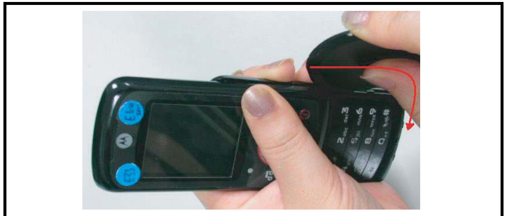
Figure 9. Removing the Lower Housing Cover
