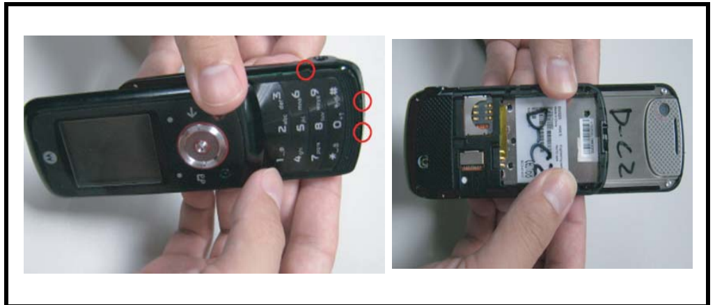
Figure 11. Replacing the Lower Housing Cover
