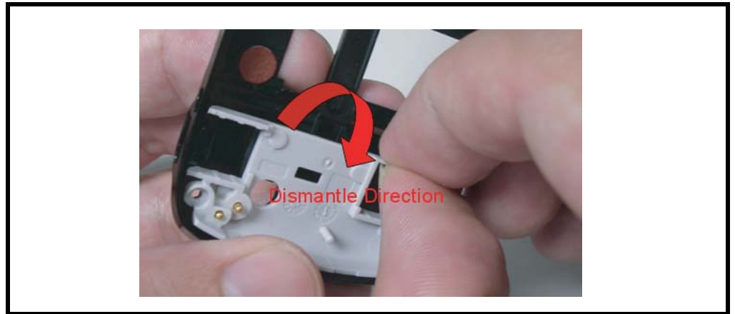
Figure 40. Remove the audio jack
