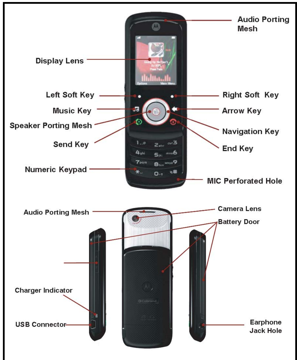
Figure 1. EM325 Telephone Controls Locations
