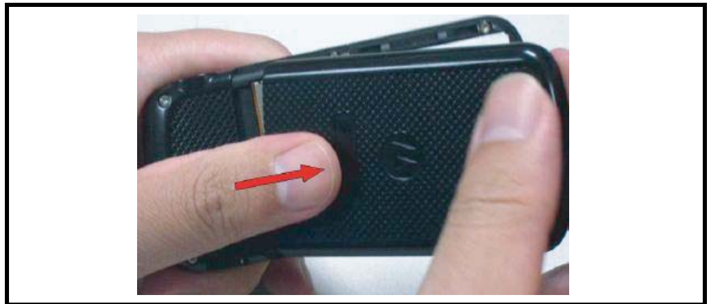
Figure 3. Removing the Battery Door
