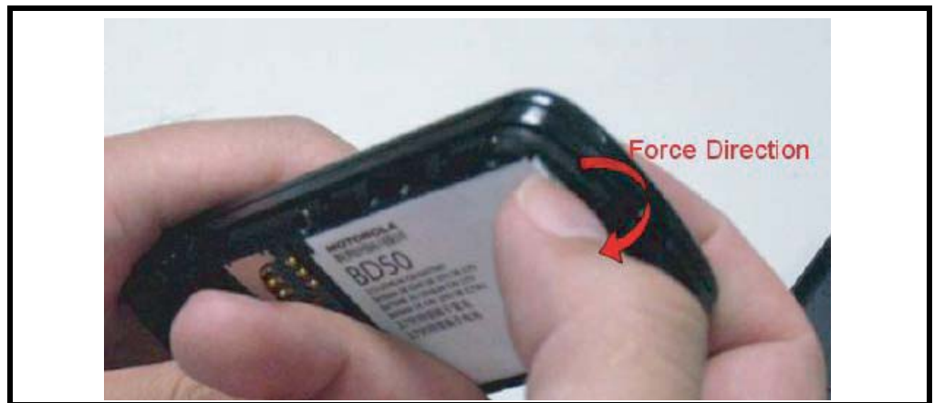
Figure 5. Removing the Battery
