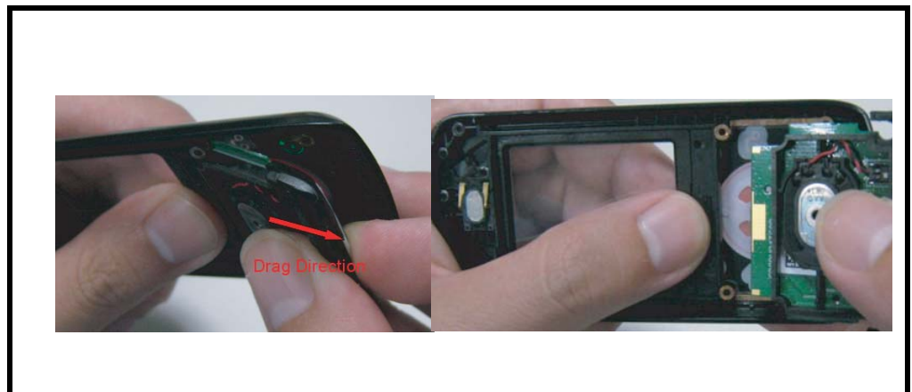
Figure 31. Removing upper PCBA
