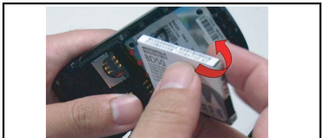
Figure 6. Replacing the Battery
