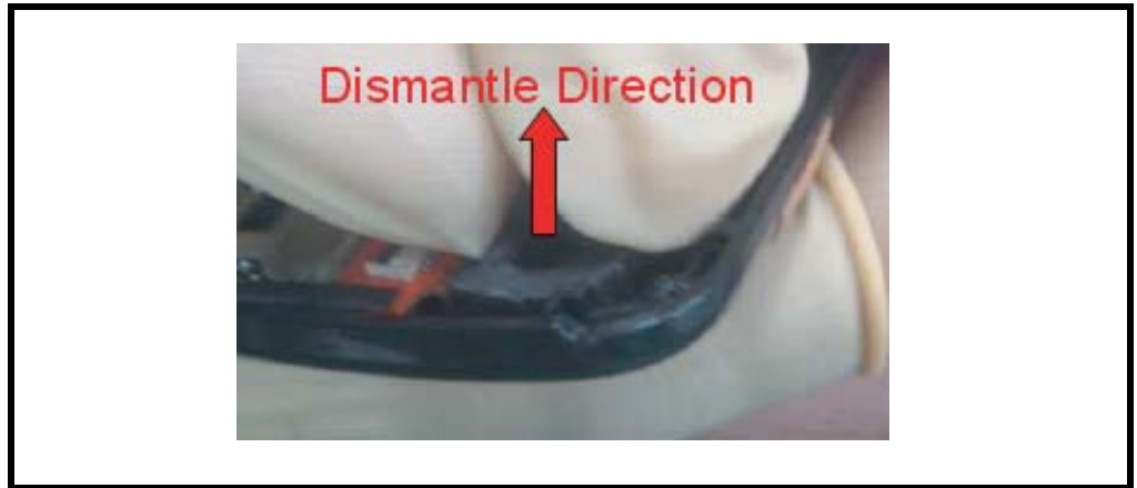
Figure 26. Removing the camera rubber
