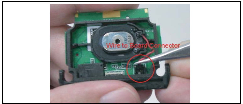
Figure 32. Removing the speaker
