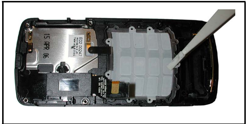
Figure 20. Removing the Keypad
