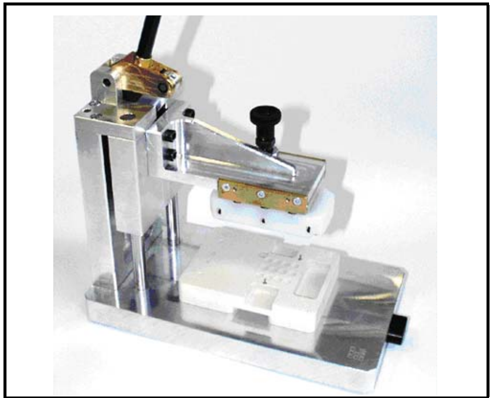
Figure 28. Z6 EL Alignment and Press Tool
