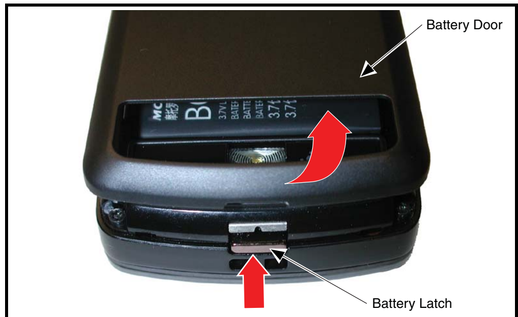
Figure 5. Removing the Battery Door
