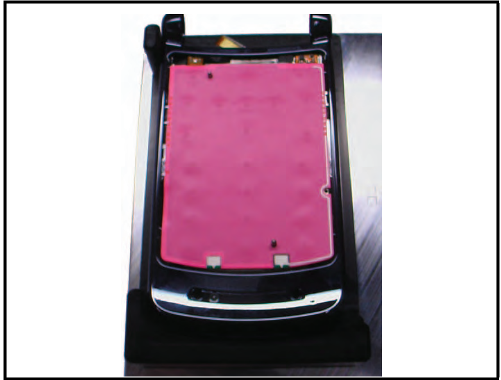
Figure 47. Front Housing Assembly in the Service Fixture
