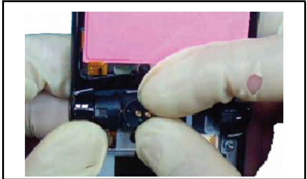
Figure 56. Installing the Vibrator Assembly
