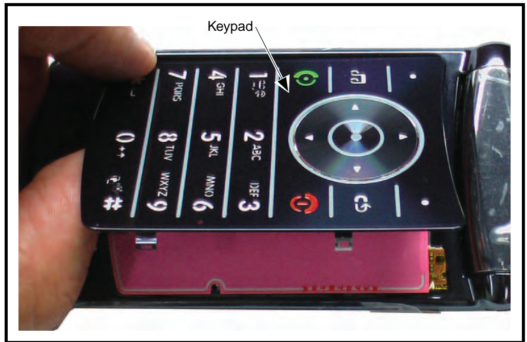
Figure 27. Placing the Keypad into the Front Housing
