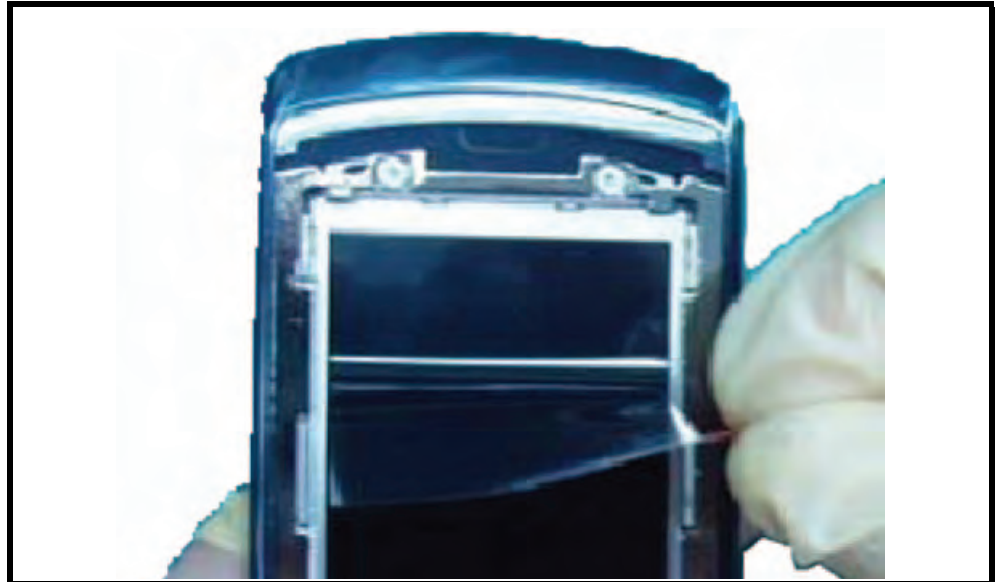
Figure 73. Removing the LCD Liner
