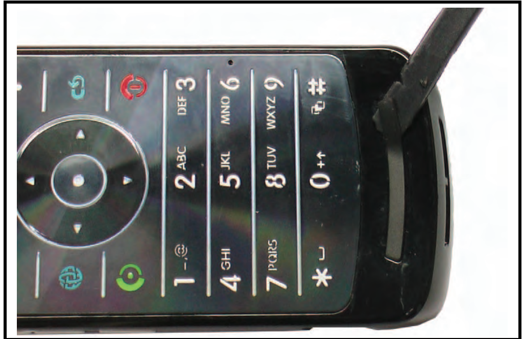
Figure 5. Removing the Bumper
