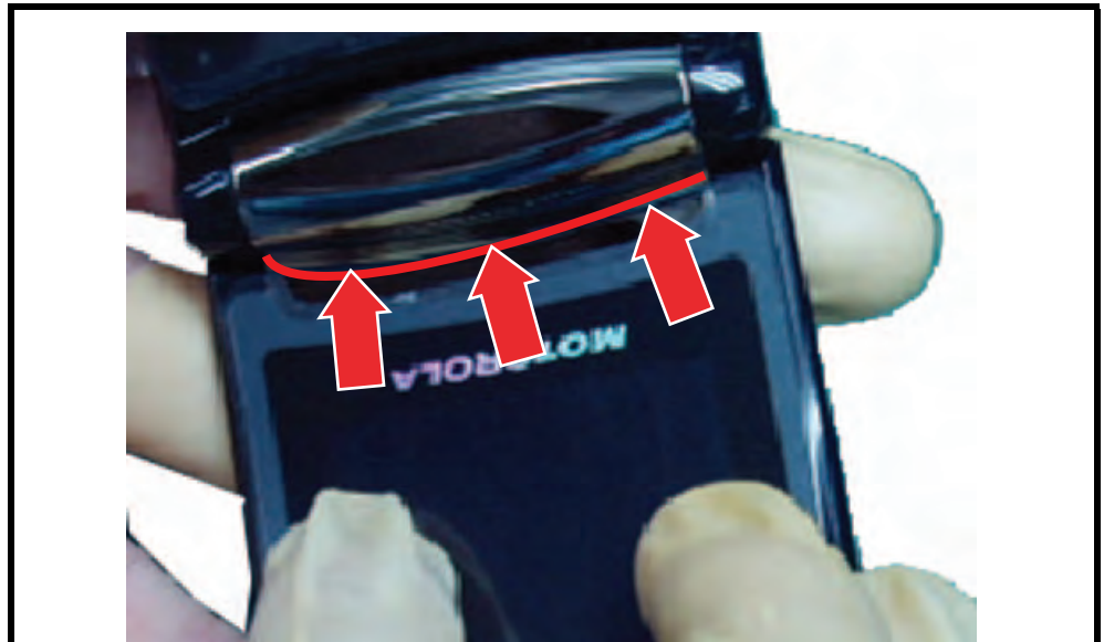
Figure 74. Attaching the Main Lens
