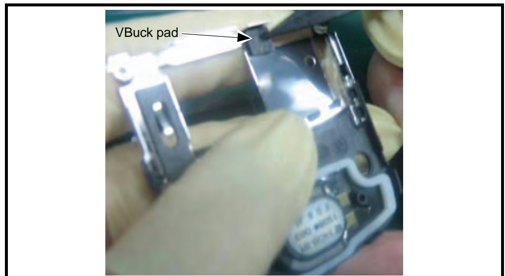
Figure 15. Installing Vbuck Pad in the Rear Housing
