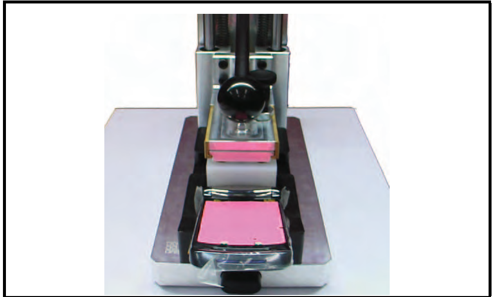
Figure 75. Pressing the Main Lens
