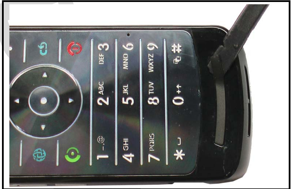
Figure 5. Removing the Bumper
