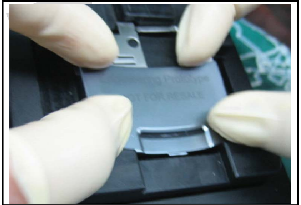
Figure 11. Attaching the Rear Housing Assembly
