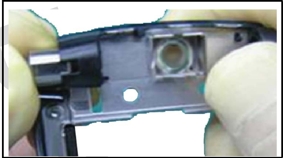
Figure 40. Removing the Lanyard Sleeve
