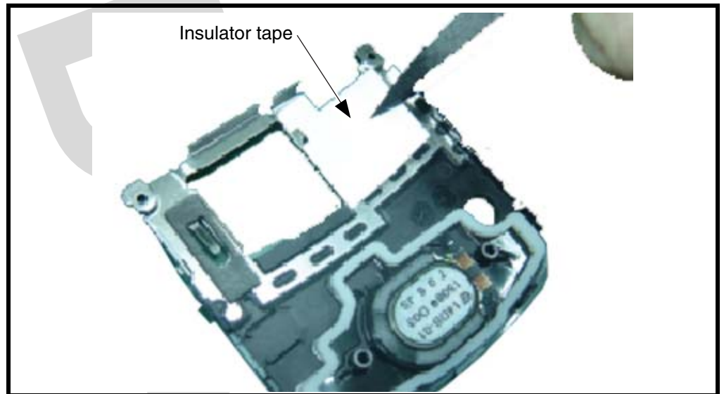
Figure 14. Installing the Insulator Tape in the Rear Housing
