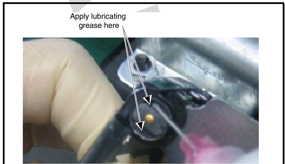
Figure 48. Lubricating the Flip Hinge
