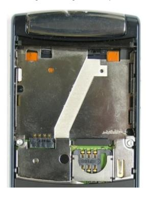
The root cause of the missing or damaged label seems to be that Customers did not understand the use of the latch at the Battery Insulator Tape.
