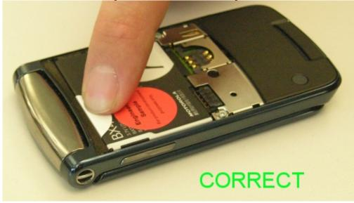
3. Make sure that the latch is hidden under the battery door
