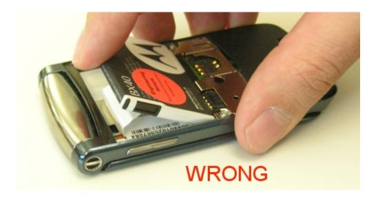
2. Bent the latch after battery insertion flat to the battery
