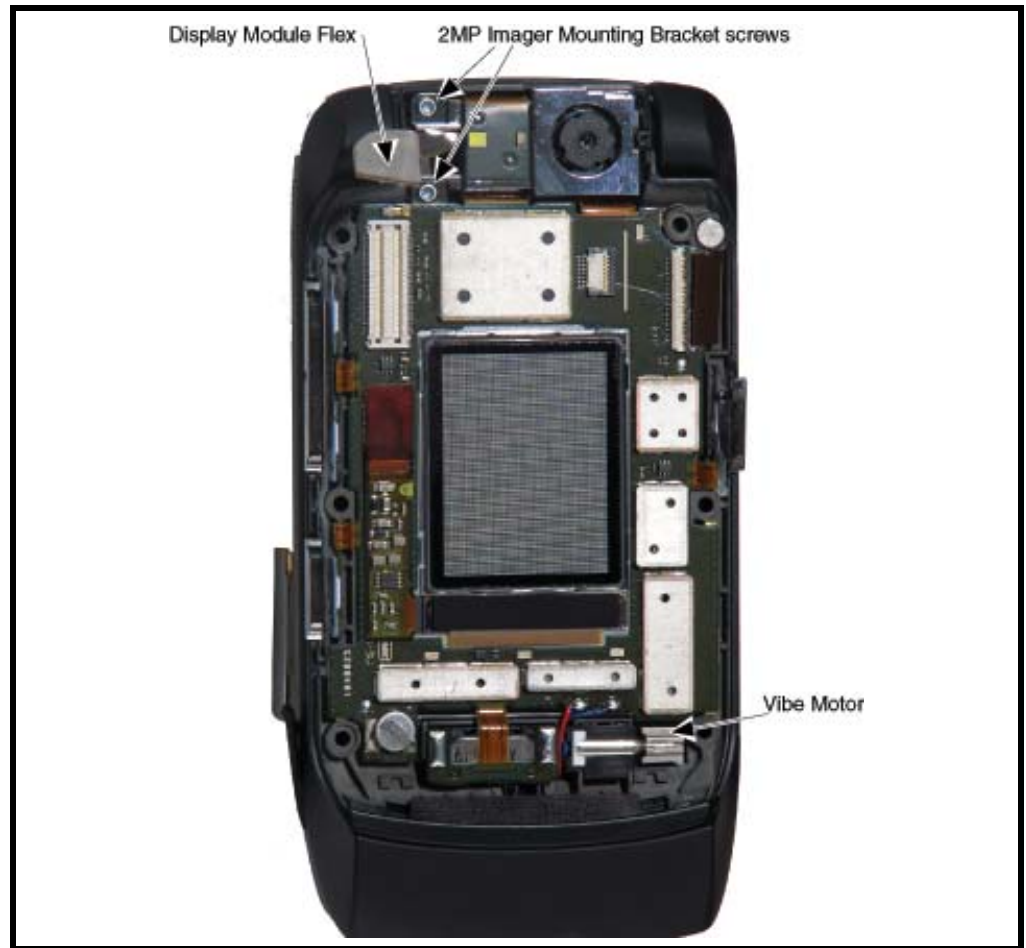
Figure 12. Display Module Assembly Flex Connector
