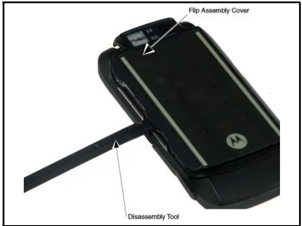
Figure 9. Separating the Flip Assembly Cover
