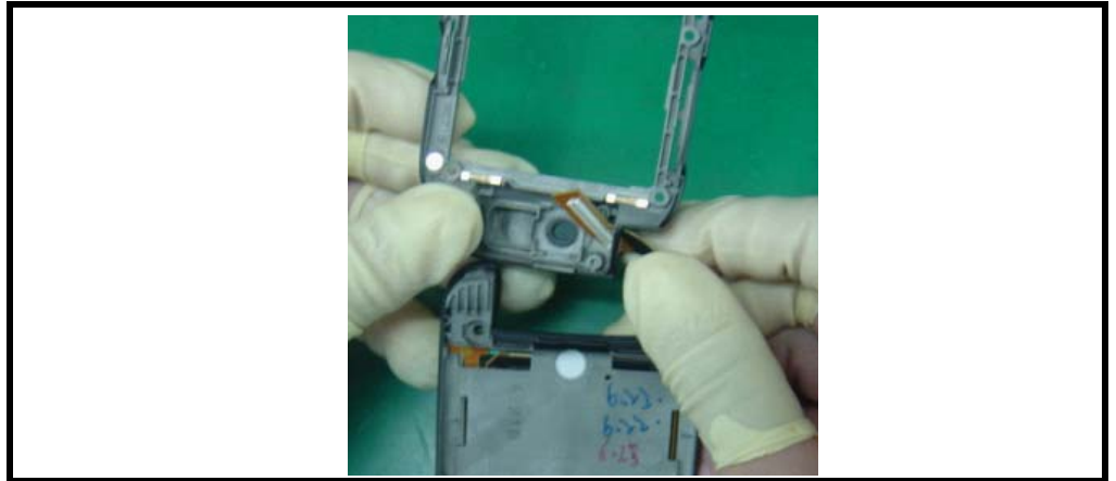
Figure 19. Removing the Flex Cable from the Flip Hinge Assembly
