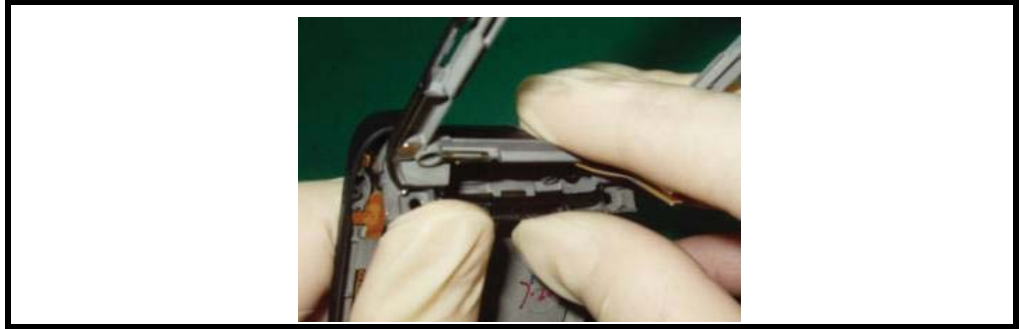
Figure 17. Removing the Flip Hinge Assembly
