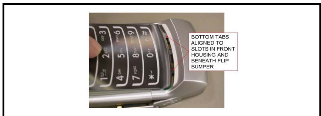
Figure 15. Removing and Replacing the Keypad Assembly
